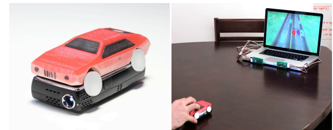
Figure 16. We created a highway racing game where users can translate a car prop on the tabletop to control their in-game car.
