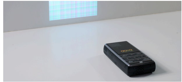
Figure 5. The AAXA Technologies L1 projector emits a focus-free image using an LCOS panel and laser light.
