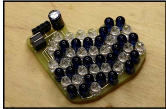
Figure 4. Light source of 24 red (clear) and 24 infrared (dark) high-output light emitting diodes.
