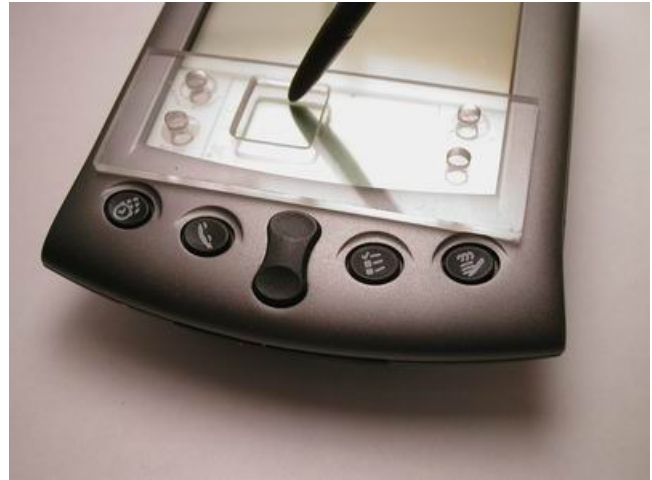
Figure 1. A Palm PDA with an EdgeWrite template over the text input area. A user makes all letters, numbers, and punctuation inside the square hole by moving the stylus along the edges and across the diagonals of the square. Small holes in the template provide access to the four soft buttons on the Palm.
